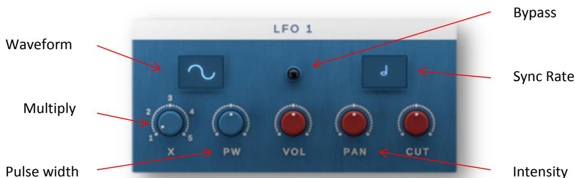
**Waveform:** Set the Waveform from SINE, SAW, TRIANGLE and RECTANGLE.
