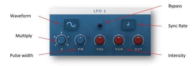
Waveform: Set the Waveform from SINE, SAW, TRIANGLE and RECTANGLE.
